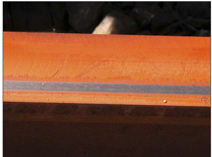
Figure 4. A range of narrow, 3/8-inch contact bands was used to vary wheel-tread contact on tangent track.
