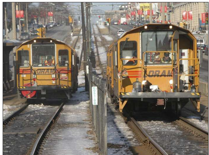
Figure 3. ARM used a pair of Loram L-Series grinders to meet MBTA's needs.
